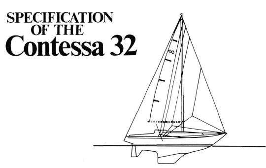
Length overall32 feet9.75 metresLength water line24 feet7.31 metresBeam9 feet 6 ins2.98 metresDraft5 feet 6 ins1.65 metresLead Ballast4,500 ilbs2,045 kilosWindward sail area562 sq feet52.2 sq metresIOR Rating22.5 feet — 23 feet
